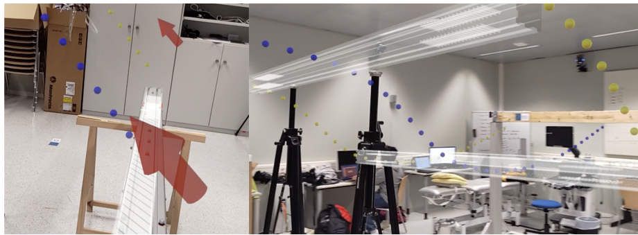
Fig. 1: Visualizations used for guidance of the movements. On the left side, the arrow is positioned above the real bar. On the right side, we can see the trajectory dots and ghost bars.
