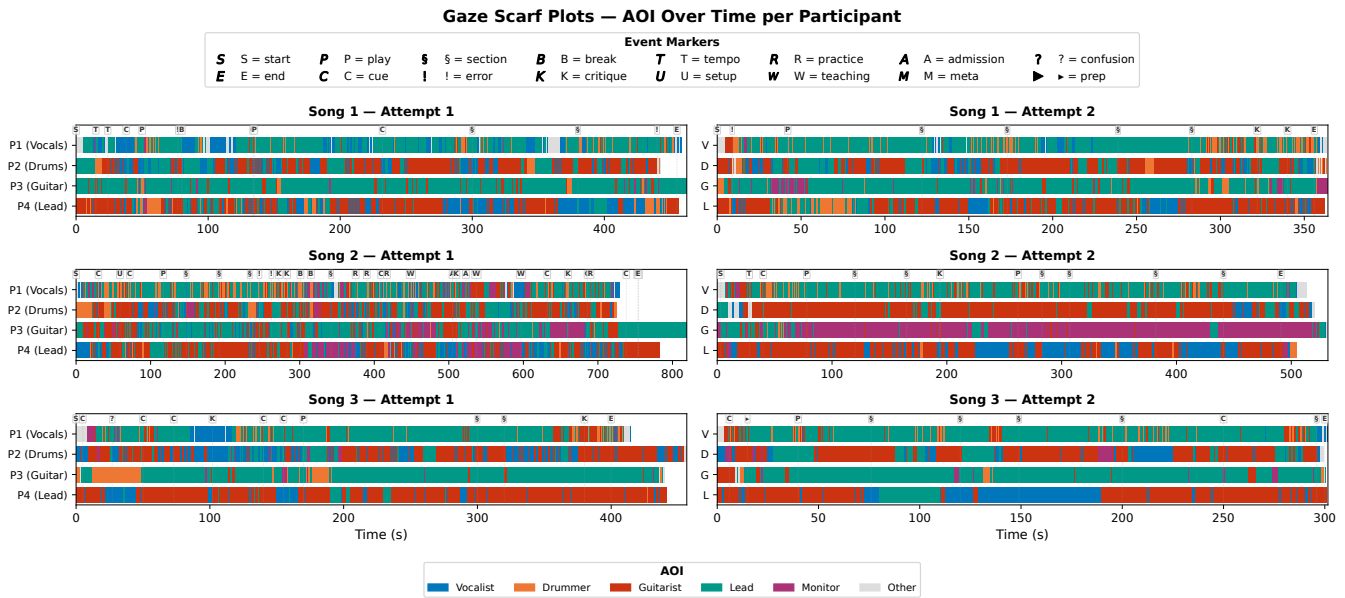
Figure 5: Scarf plots of sequential AOI fixation targets for all six sessions (3 songs × 2 attempts). Each row is one participant; colored segments indicate the fixation target, with grey for unclassified fixations. Vertical markers denote events (stops, teaching, count-ins). S2 A1 shows fragmented scanning with frequent stops; S3 A2 shows stable, sustained attention.
