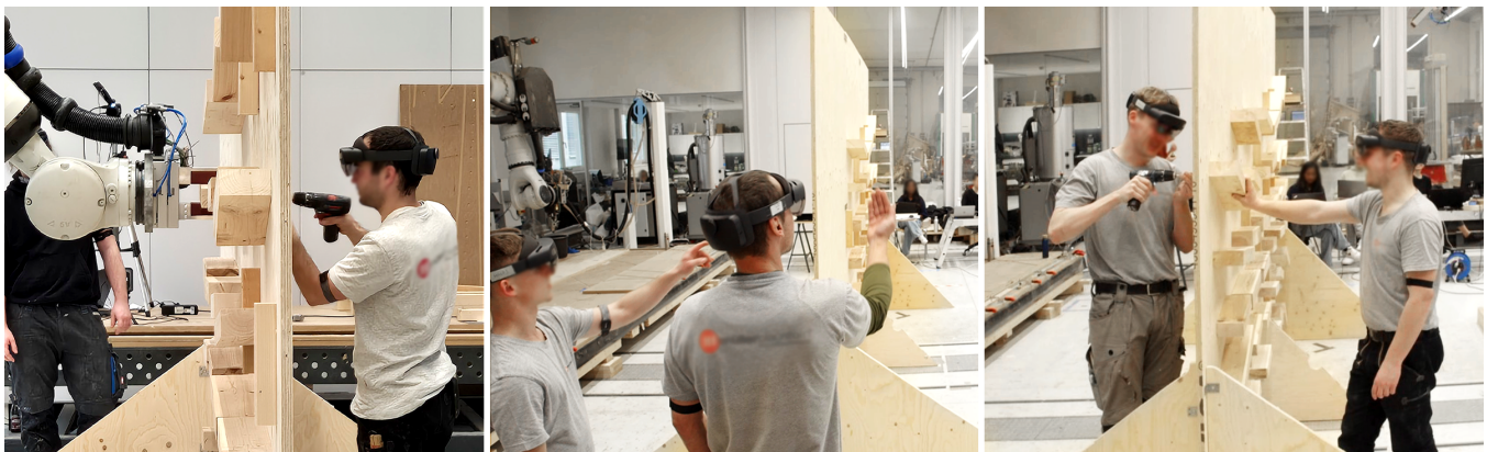
Figure 1: Photos of the Study. Left: user inserting screws while the robot holds the beam. Centre: two users discussing how to intervene in the robotic task. Right: two users collaboratively assembling a timber beam during human-human collaboration.
