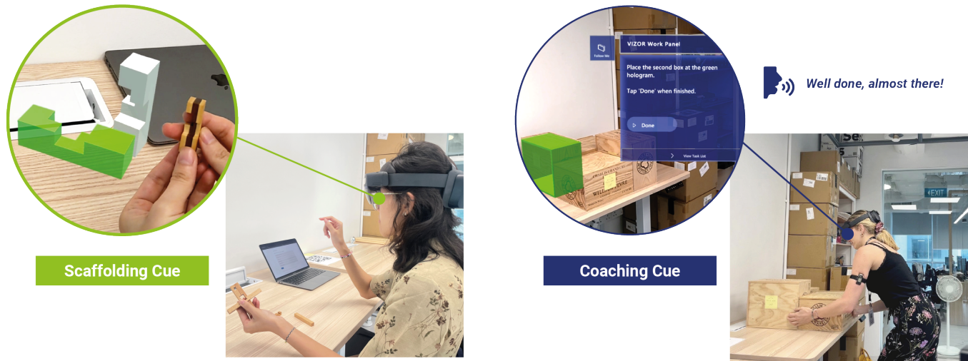
Figure 4: Scaffolding cues were implemented for the cognitive tasks where users assemble interlocking joints (left). The image shows the active cue (green element), which has been moved away from the main structure, and the inactive piece in light grey. Coaching cues were implemented for physical tasks where users assemble box clusters (right). The image shows the location of the box placement in green, with a task panel to confirm the completion of the placement.
