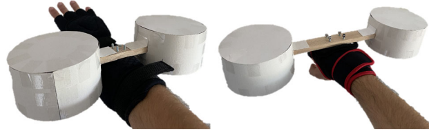
Fig. 2 The paper mockup used in our form factor pre-study. Left/right: attached to the wrist/hand. This figure consists of two images showing the paper mockup used in our form factor pre-study. In the first image, the paper mockup is attached to the user's wrist and in the second to the hand, using two different fitness gloves
