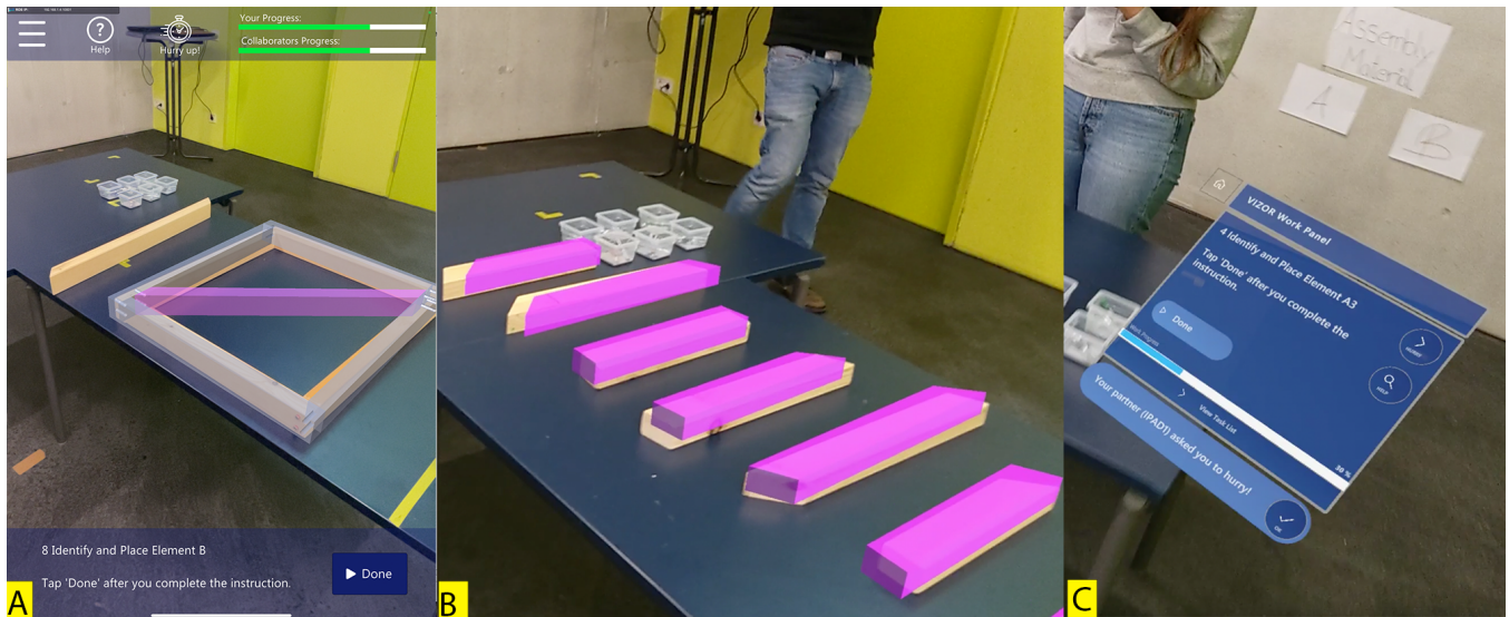
Figure 2: A: Interface of the HHD and assembly task structure. B: Timber sticks positioned in the sorting task. C: HHD interface showing one of the predefined messages from partner.
