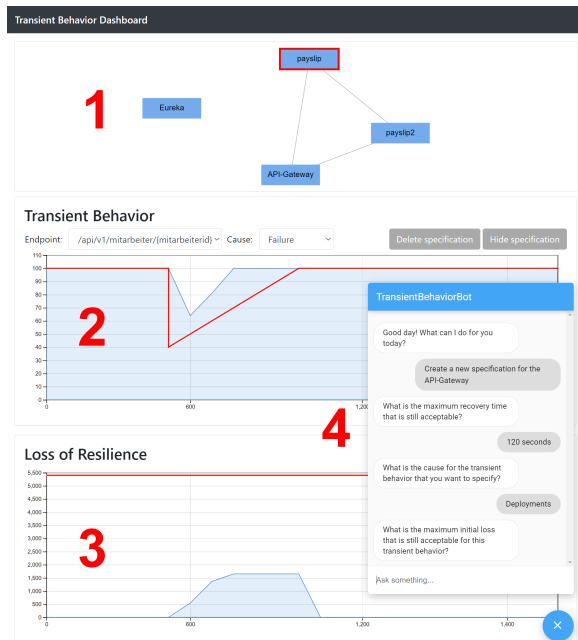
Figure 2: TransVis includes visualizations for a system’s (1) architecture, each service’s (2) transient behavior and (3) loss of resilience, and a (4) chatbot.
