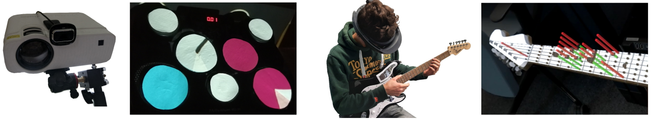
Figure 1. The two augmented reality setups we explored: Left: Using a projector on a tripod, we display visualizations on the pads of a drum kit. Right: A user wearing an optical see-through AR headset sees visualizations on a guitar's fretboard.
