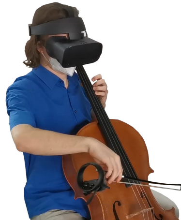
Figure 2: We currently track position and orientation of the bow through a VR controller fixed to it.
