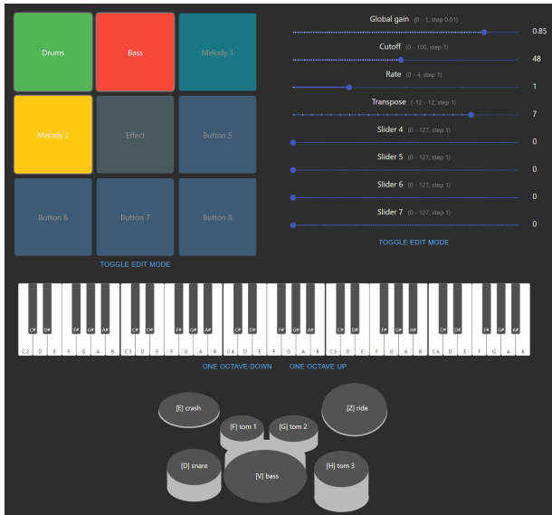
Figure 1. Our design allows live coders to perform certain actions through a visual interface to influence the behavior of code without edits. Commands are transmitted over MIDI from a web app to Sonic Pi.
