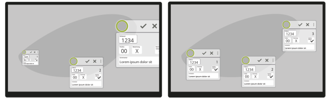
Figure 6: Perspective projection of UI elements with distance-dependent visual size (left). Drawing overlays and annotations as parallel projection results in equally sized interface elements (right).
