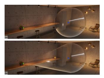
Figure 2: The glass surface represents all possible swarm positions for the given camera location (blue sphere) and target (green sphere). Two placement options are considered: (a) Placement on a sphere, where the swarm maintains a constant distance of 1m to the camera; and (b) Placement on sphere+cone, where the swarm can leave the spherical surface and fly towards the target, which is at an approx. distance of 3.5m. 3D scene from Unity Technologies<sup>4</sup>.
