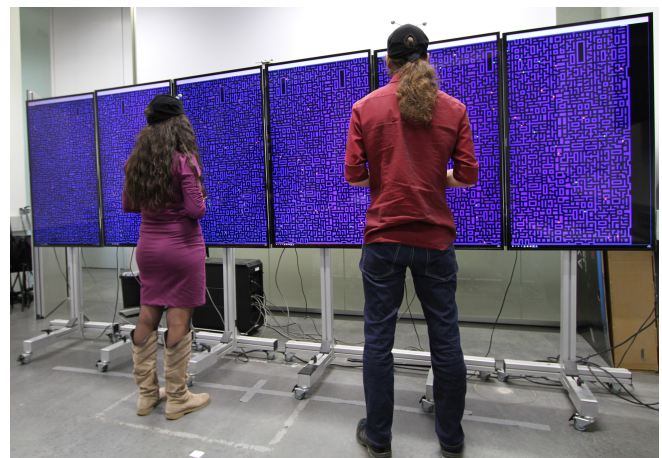
Figure 2. A player pair standing in front of the LHRD engaging in Pac-Many while wearing the mocap beanie hats for position tracking.
