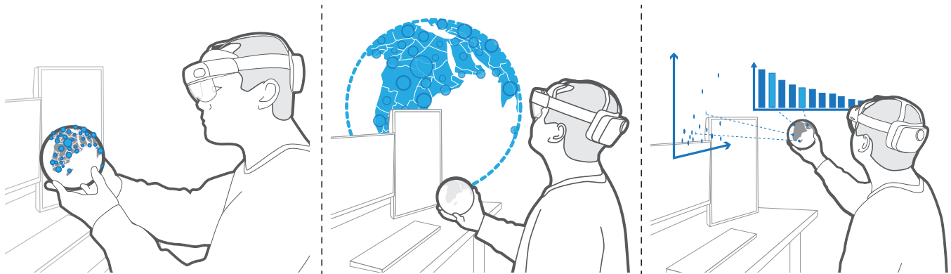
Figure 1: We envision three general categories of how AR geospatial data visualisation can be supported by physical, tangible globes. The augmented globes category (left) puts information space on and around the tangible globe. The tangible globe input category (middle) utilises the spherical form-factor and tactility of the tangible globe to control virtual information space. The complex interplay category (right) combines the two, creating distributed information spaces. Note: virtual elements are illustrated in blue throughout the paper.
