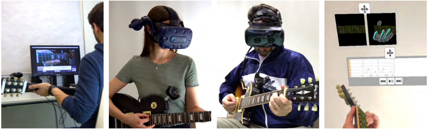
Fig. 5: Participants in the first evaluation used (left) the desktop magic mirror display or (center left) the HTC Vive Pro head-mounted display. Instead, the second evaluation used (center right) the Varjo XR-3 head-mounted display. Alternatives to augmented guidance included (right) a tablature view and a virtual mirror.
