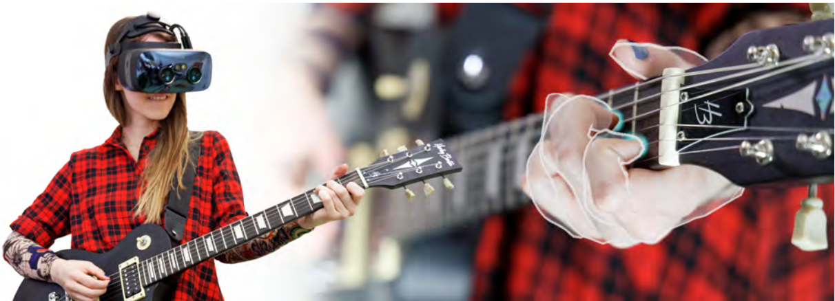
Fig. 1: We present a system that can visualize automatically generated guitar tutorials using two alternative AR display modalities: Users can view augmented instructions using a video see-through head-mounted display or a desktop display.
